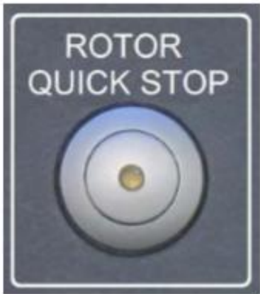
Figure 5.6: Rotor Quick Stop Button on the Back Panel of the MAS III
